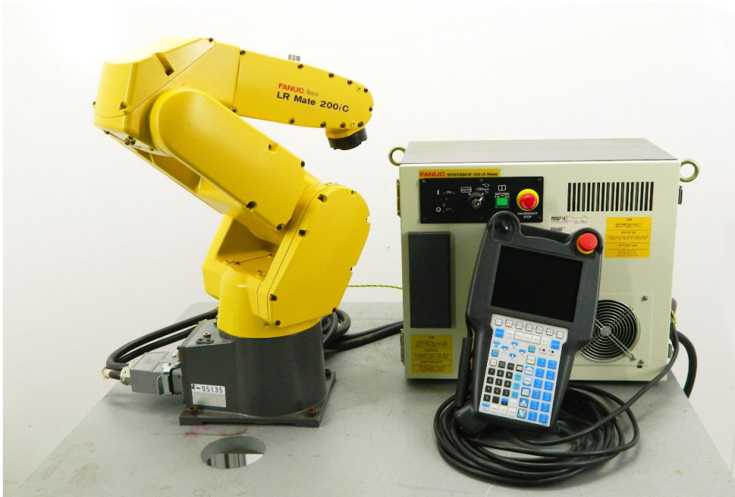
Rys 1. System sterownia z manipulatorem LR Mate 200iC
